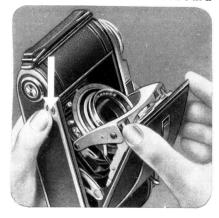
camera to open it. Pull down the baseboard by its two corners until the struts click into position. It is then ready for use.
