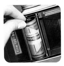
under the film winding knob holds the empty take-up spool. If it is in the other chamber, remove it and change it over (see bottom of page 14).
