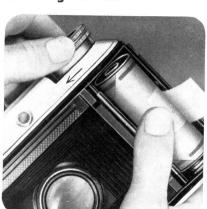
www.orphancameras.com Close the baseboard (see page 4) and wind the film winding knob in the direction of the arrow until the whole of the film has been wound on to the take-up spool. Through the film window you can watch the backing paper move past.
